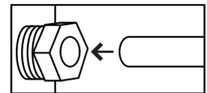
2. Insert tubing into fitting.
