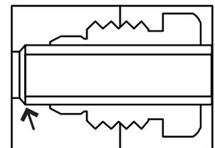
4. Hold tubing against shoulder and tighten nut.
