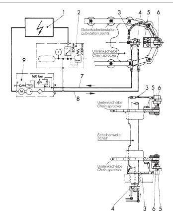
Electrical control cabinet Pressure storage unit consisting of: Accumulator Pressure gauge Pressure switch 180 bar Pressure relief valve 200 bar 3. Flexible hose connecting the
