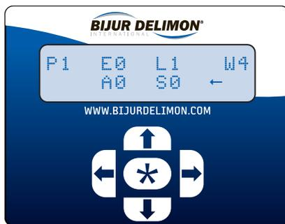
P1 - PRESSURE SWITCH ENABLED
