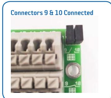
This image shows the position of the connectors when terminals 9 and 10 are connected.
