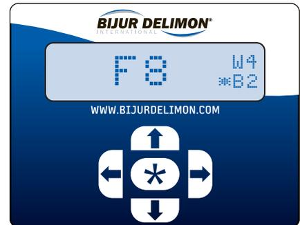
AIR PRESSURE SWITCH FAULT SCREEN
