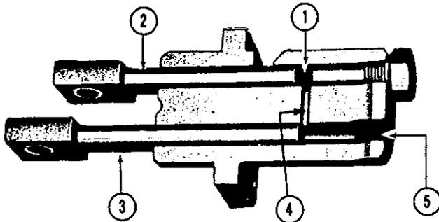
C. Main piston (2) continues right, forcing lubricant from main chamber (1) through discharge port (4) and outlet (5) to system supply line. Valve piston (3) continues left.
