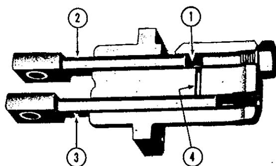
F. Main piston (2) continues left preparatory to opening lubricant port to main chamber (1). Valve piston keeps discharge port (4) closed. Sequence repeats when pistons reach original positions.
