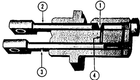
B. Main piston (2) moves right, exerting pressure on lubricant in main chamber (1), as valve piston (3) moves left to open discharge port (4).
