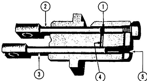
E. Main piston (2) moves left, creating vacuum in main chamber (1), while valve piston (3) continues right, blocking discharge port (4) and outlet (5) to system supply line.
