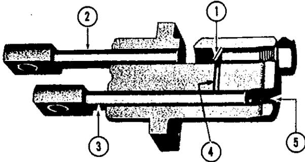
A. Lubricant enters main chamber (1) from reservoir when main piston (2) reaches extreme back stroke position. Valve piston (3) blocks discharge port (4) and outlet (5) to system supply line.
