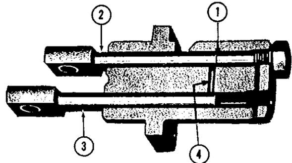
D. Main piston (2) reaches extreme forward stroke, exhausting all lubricant from main chamber (1). Valve piston (3) moves right to close discharge port (4).
