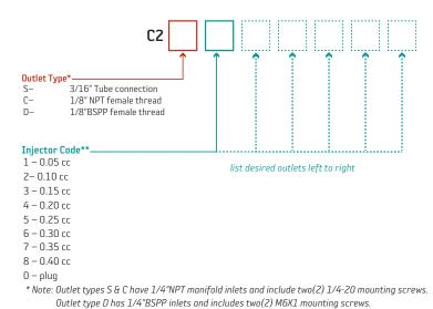
\*\* Injectors are mounted on top and facing forward in manifold.
