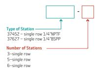
Note: 1/4BSPP is equivalent to "G1/4" female threads. Copper washers required to seal, p.n.35010.
