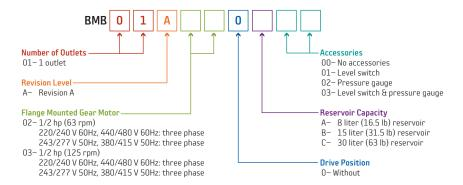
The BM-B Lubricator features a smart part number ordering system, where you can tailor the pump to meet your needs. First, choose the number of outlets, revision level, flange mounted gear motor, drive position, reservoir capacity and accessories you need. Then, put the numbers into the corresponding squares in the easy-to-use grid. You now have the customized part number.
