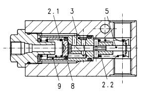
The main line is relieved. The compression spring (item no. 2.2) presses the control piston (item no. 5) into its right final position. The delivery piston (item nos. 8 and 9) is also pressed into its right final position by the compression spring (item no. 2.1).
