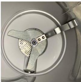
A feed insert with scraper, which rotates while the pump is running, is installed in the reservoir base. The rotation speed corresponds to the piston speed (max. 10 rpm). The scraper ensures regular mixing of the lubricant and prevents deposits (when grease is used) on the inner wall of the reservoir, which can occur especially if the lubricant remains in the reservoir for a long time.
