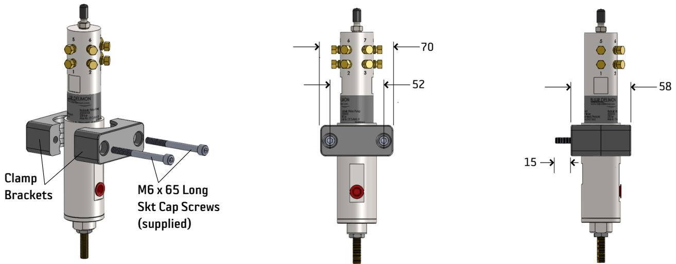
Oiler may be bolted directly to pre-tapped M6 holes (@52 centres) on the machine OR more usually, secured through a bulkhead (with  $\Phi 6.5$  drilled holes @ 52 centres) and fastened with nuts and washers. The screws supplied enable mounting with either option.
