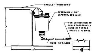
Use for priming any Bijur Delimon lubricating system after installation.
