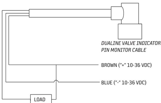
BLACK (OUTPUT; 10-36 VDC, 100mA MAX LOAD)
