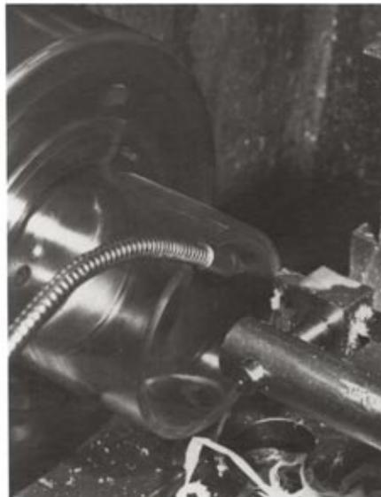
FluidFlex Jet B-101 delivers coolant resulting in lower temperatures during turning operation and, thus, higher productivity and better part finishes.
