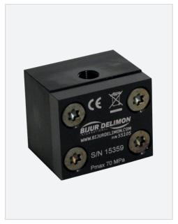
An accurate oval gear mechanism that incorporates two magnets into one of the nylon oval gears. The body incorporates a reed switch, which senses the magnet passing. Lubricant entering the 55105 causes the gears to rotate. Each pulse equates to an approximate displacement of 0.040 cu. in. (.65 cc). The monitoring of the 55105 is done with any PLC or the dedicated DS405 Controller. The feedback from the 55105 will assure that lubricant has reached the inlet of critical lubrication points.
