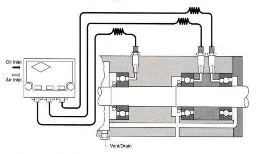
Typical high-speed spindle installation.
