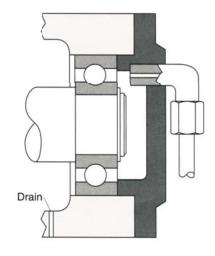
Drain ports prevent lubricant back-up in housing.
