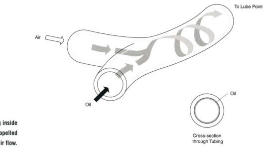
Oil travels along inside wall of tubing propelled by air flow.
