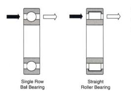
Delivery of air/oil through the bearings for effective lubrication.
