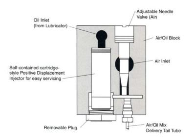
Bijur's HyperFormance Air/Oil Lubricating System utilizes an air/oil positive displacement injector block to deliver a precise amount of oil into a controlled air flow. Air propels the oil droplets along the inside wall of small bore tubing until it reaches the lubrication point. The tubing length stretches out the flow of lubricant so that a continuous flow arrives at the nozzle.
