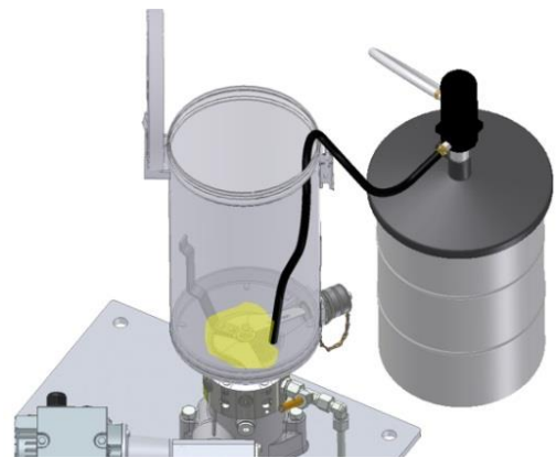
Example of filling using the reservoir lid
