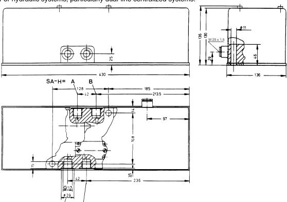
When using SA-H as 2/2-way valve with port A, 1 port B has to lead back into the reservoir and close the opposite one.
