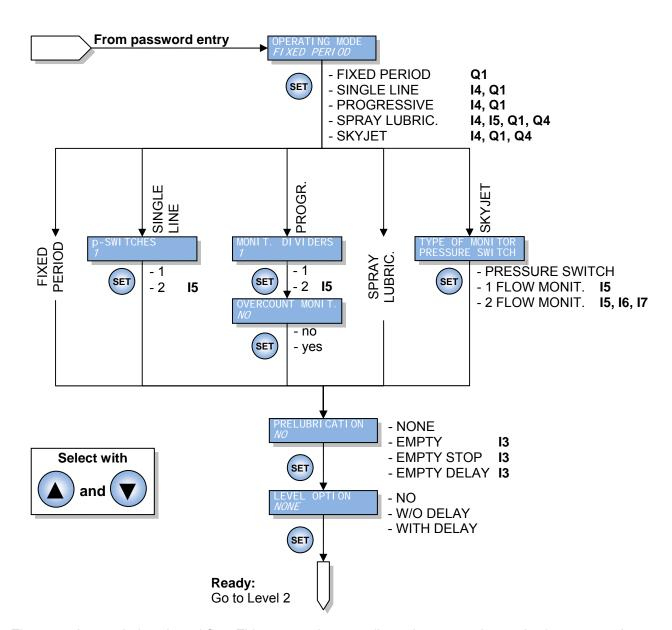
The operating mode is selected first. This causes the controller to jump to various selection trees and call up only the basic settings for the selected mode.
