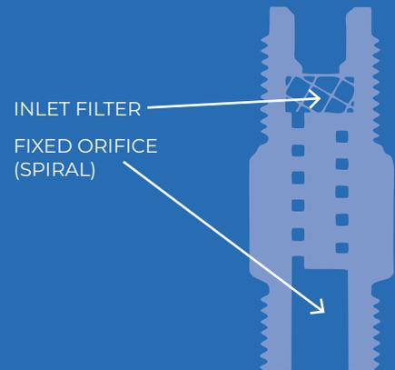
Resistance fittings may either be direct mounted at the bearing or off-set from the point of lubrication. When direct mounting a resistance fitting into a bearing, either straight units or tee units are used. They assure the most rapid transfer of oil.
