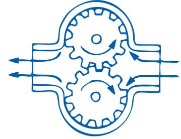
Normally, continuous lubricators are rotary-driven gear pumps which are fully submerged in oil at the bottom of a reservoir and protected by a coarse metal suction screen. Operating pressure is limited to 100 or 200 psi by a built-in relief valve. Discharge from the pump is controlled by a bypass valve. Several size reservoirs (plastic or metal) are available. Also available are pressure monitors and low level oil switches.
