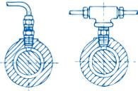
For drip-feed lubrication – cams, gears, chains, etc. – a junction unit is screwed into a standard junction block in the distribution line.
