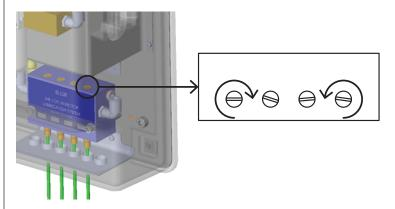
Note: To adjust the needle valve a short slotted head screw driver is required.
