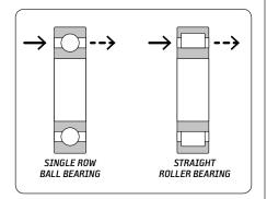
Bearings dynamics affect the delivery method of how air/oil flows through the tubing. Air/Oil deliveries must flow unimpeded through the bearing for successful lubrication. Always ensure a free air flow passage through the bearing element. Air restrictions and back pressure can impede proper deliveries to critical areas.
