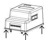
The Air-Oil Mixing Unit's cover handles are only for fitting and removing the Air-Oil Mixing Unit cover.
