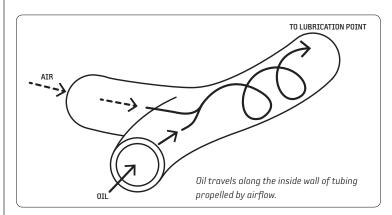
Air expansion at the nozzle outlet generates a controlled spray for efficient bearing lubrication. A wide selection of injector rates combined with individually adjustable air valves provide specific air/oil deliveries to maintain thin lubricant oil films to each high-speed anti-friction bearing or other surfaces.
