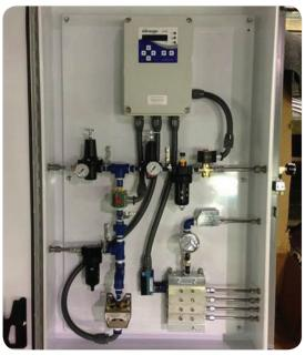
Automatic Grease System in Enclosure
