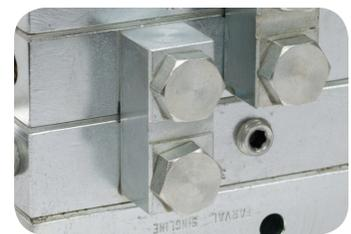
"C" Porting on face of valve section
