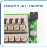
This image shows the position of the connectors when terminals 9 and 10 are connected.
