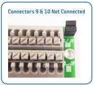
This image shows the position of the connectors when terminals 9 and 10 are not connected. This is the default position.
