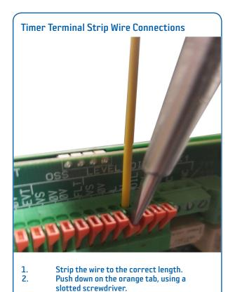
Insert the wire fully, release the orange tab. Pull the wire to ensure it is inserted
