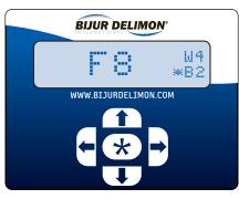
AIR PRESSURE SWITCH FAULT SCREEN
