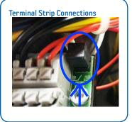
The terminal strip has a built in option to connect pins 9 and 10, this enables a common wire to be used for both the level switch and pressure switch if required. The status of the switch can then be monitored via pins 8 and 11.
