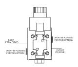
WHEN USED AS A ZONE CONTROL VALVE NORMALLY OPEN POSITION
