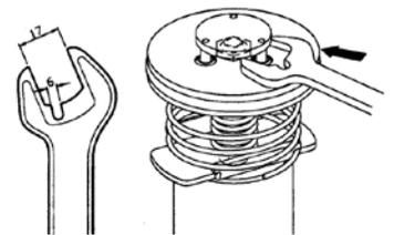
Remove inverting set with 17mm wrench
