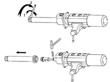
Unscrew tube assembly, remove
